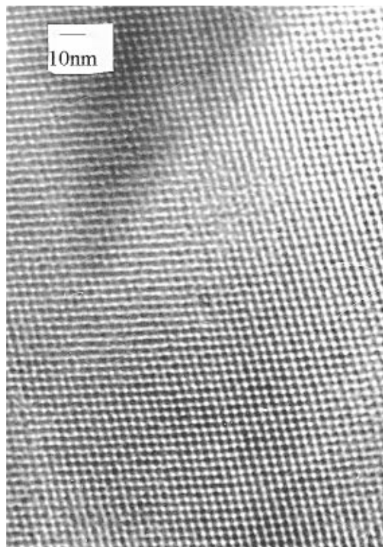
Figure 2. Representative HREM image of calcined MCM-48 showing the mesopores on the (110) cubic plane. This image was obtained with a JEM-200CX transmission electron microscope operating at 200 kV from a thin section prepared by ultramicrotomy.
